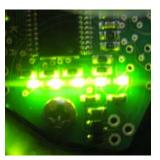
The Scurion<sup>®</sup>-lamp has an LED bar, which mostly displays battery charge status.
